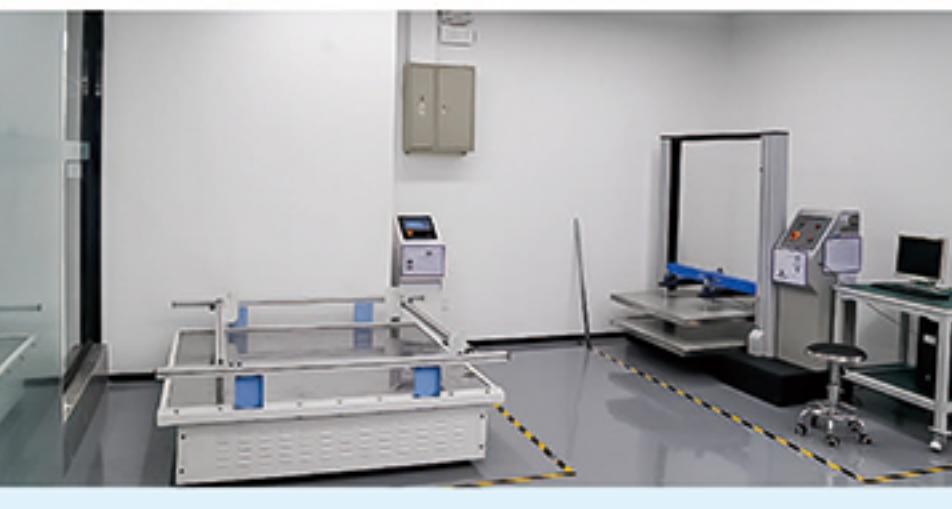
Simulated transport vibration testing
