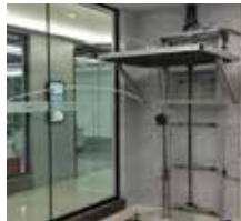
IP Waterproof Test Machine
